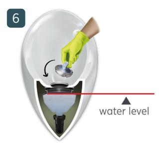
Fill the water to the point of overflow and insert the cover.
